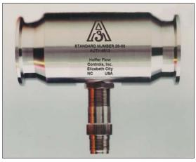
Note: Turbine meter must be installed with pickup coil pointing down to ensure proper cleanability according to the 3A standard.
