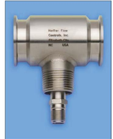
**Note:** Turbine meter must be installed with pickup coil pointing down to ensure proper cleanability.
